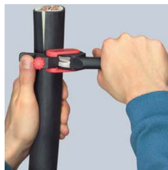
Turning the tool for circumferential cut
